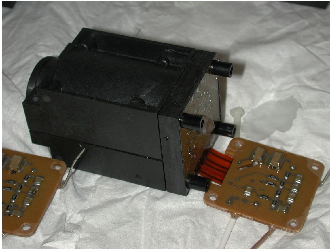
Conformal coating of the PM base after cabling
