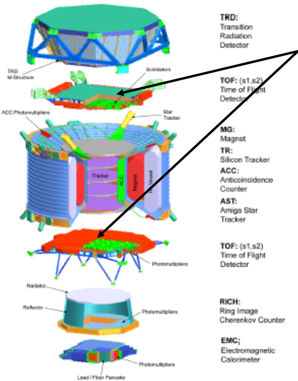
The second element to complete the ‘basic’ spectrometer is the Time of Flight System (TOF)
