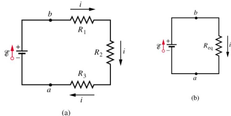
$$E - iR_1 - iR_2 - iR_3 = 0 \Rightarrow i = \frac{E}{R_1 + R_2 + R_3} = \frac{E}{R_{eq}} \Rightarrow R_{eq} = R_1 + R_2 + R_3$$
