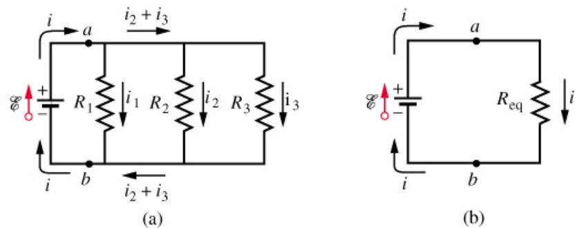
$$i = i_1 + i_2 + i_3 \Rightarrow \frac{E}{R_{eq}} = \frac{E}{R_1} + \frac{E}{R_2} + \frac{E}{R_3} \Rightarrow \frac{1}{R_{eq}} = \frac{1}{R_1} + \frac{1}{R_2} + \frac{1}{R_3}$$
