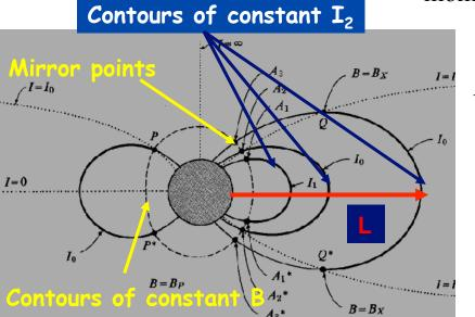
For real earth's field a new variable is defined based on dipole f<sub>D</sub>: by definition the equivalent equatorial radius, L, called McIllwain parameter, is given by LR<sub>E</sub>=f<sub>D</sub>(I,B,M<sub>E</sub>)
