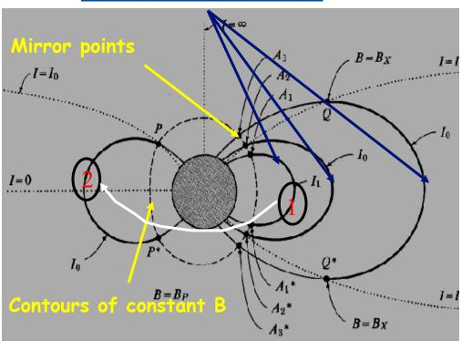
The primary use of I<sub>2</sub> is to find surfaces mapped out during bouncing and drifting. A particle initially on curve 1, with a given I, will drift on curve 2 (with the same I) and return to 1, mirroring at B<sub>m</sub> in both the hemispheres throughout the drifting. At each longitude there is ONLY one curve -or field line segment- having the required value of I. The particle will follow a trajectory made of field line segments such that I is constant.
