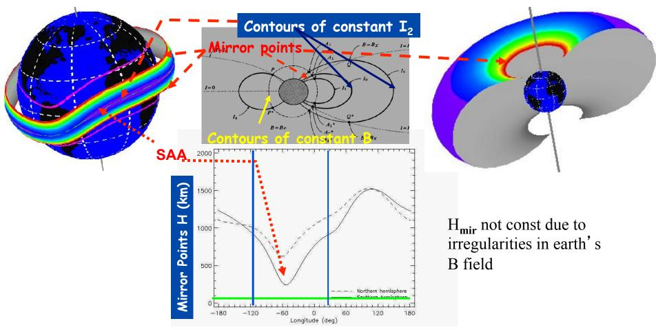
All the particles with the same invariants map out the same drift shell, i.e. are equivalent from magnetic point of view
