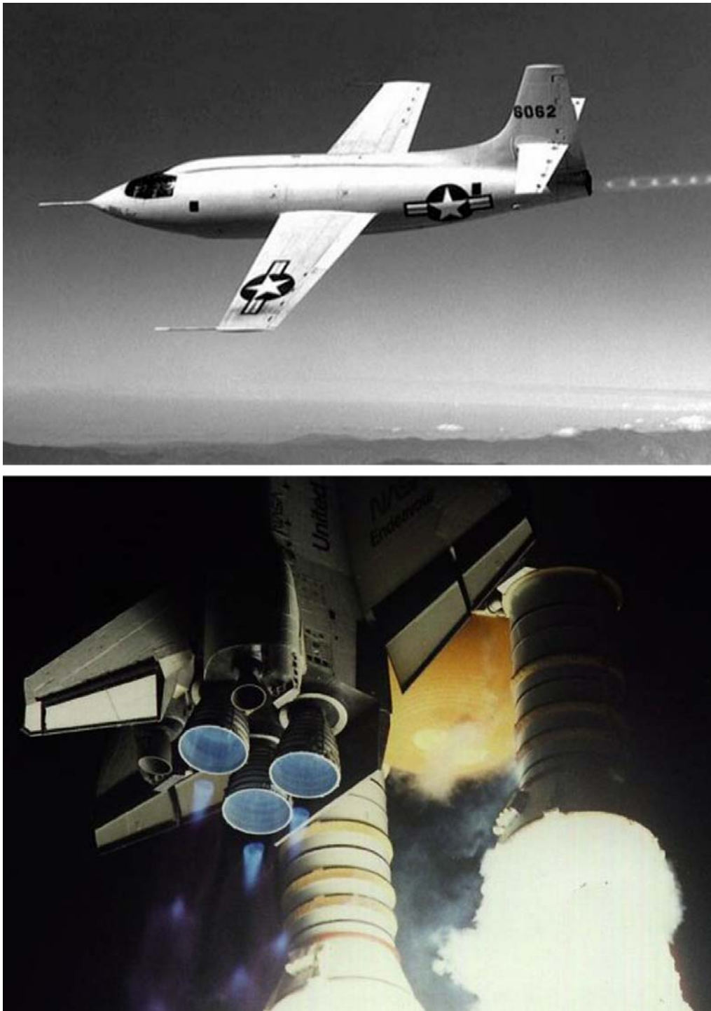
Figure 7.8: Mach Disks in the exhaust jet of the Bell X-1 rocket plane (top), and behind the three main engines of the Space Shuttle (below). Behind the Bell X-1 a series of bright 'blobs' are visible, which show the location of the series of Mach Disks. Behind the Shuttle engines, only the first Mach Disk is clearly visible, the following disks in the series are less distinct.
