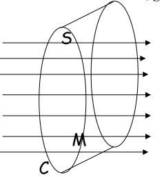
if the curve moves,  $\Phi$  changes because: (a) the B field changes in time and (b) the field lines move into or out of S
