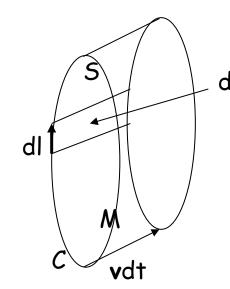
$$\mathrm{dS}_{\mathbf{u}} = \int_{S} \frac{\partial \vec{B}}{\partial t} \cdot d\vec{S} - \int_{S} \vec{\nabla} \times \vec{v} \times \vec{B} \cdot d\vec{S} \qquad \text{With the Stokes' theorem for the last term}$$
