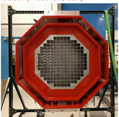
The first FBK 6x6mm<sup>2</sup> SiPM have been just installed and will equip an upgrade of the pSCT camera
