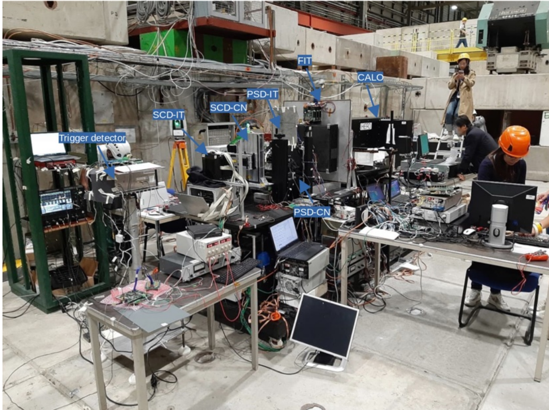
Figure (4.33) – The setup of fall 2023 HERD beam test at the CERN SPS H4 beam line.
