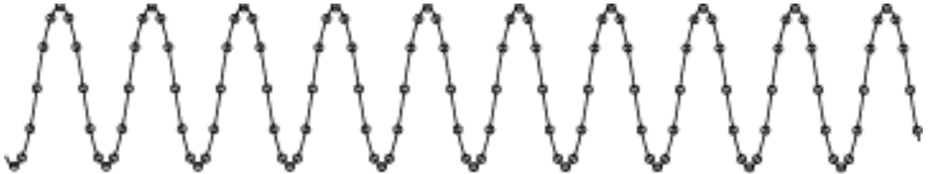
Adequately Sampled Signal
