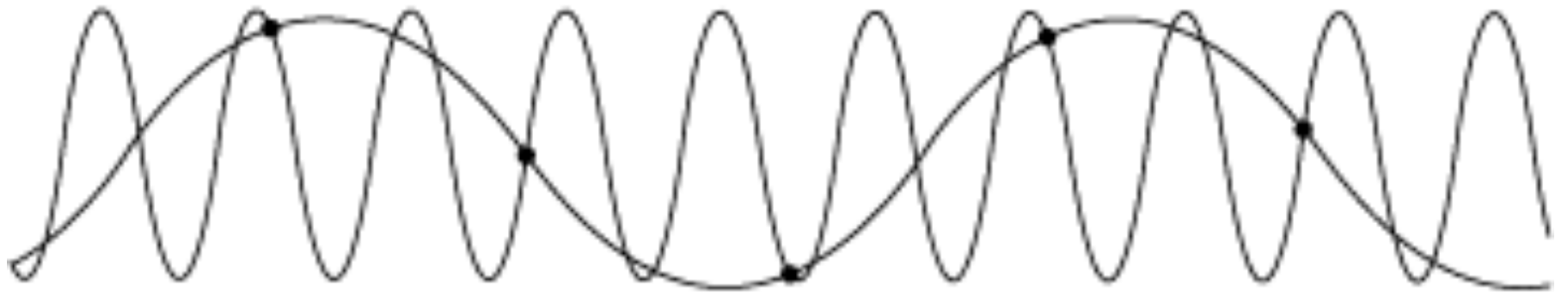
Aliased Signal Due to Undersampling
