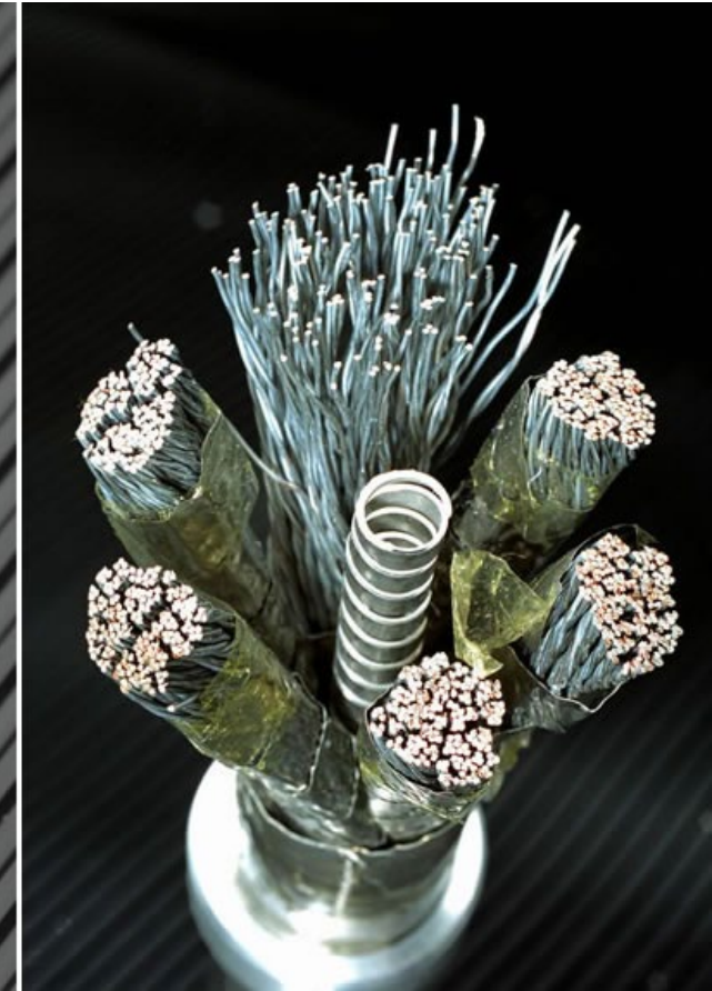
Section of the Cable-in-conduit-conductor (CICC) for the ITER magnets
