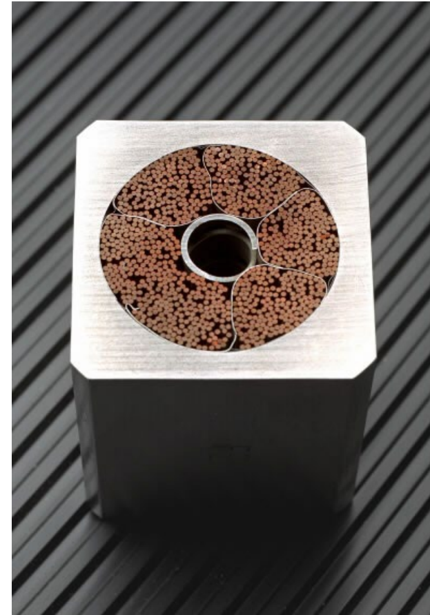
Section of the Cable-in-conduit-conductor (CICC) for the ITER magnets
