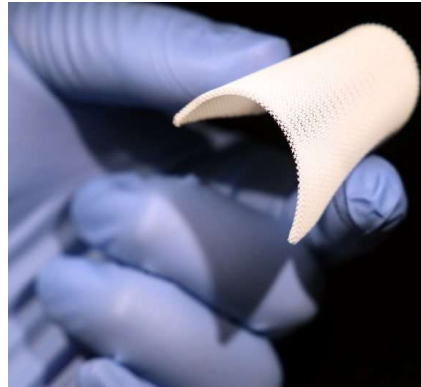
Three-dimensional printing of piezoelectric materials with designed anisotropy and directional response, Cui et al (2019)
