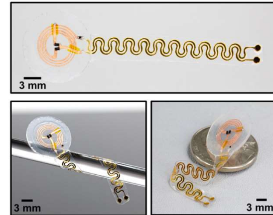
Battery-free, tuning circuit-inspired wireless sensor systems for detection of multiple biomarkers in bodily fluids, Liu et al (2022).
